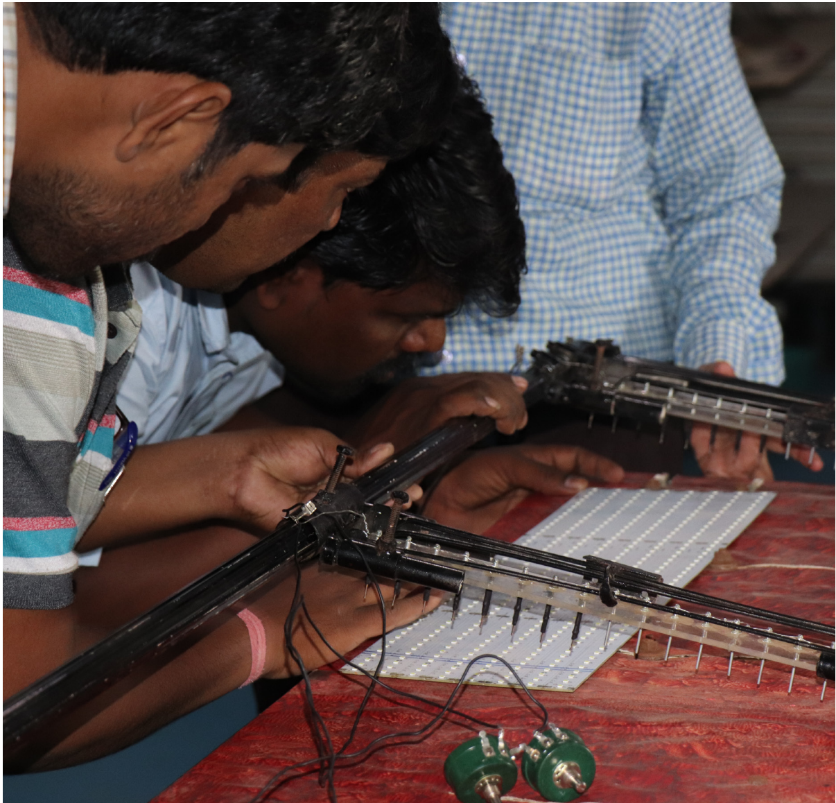
The LED testing panel developed by students for Manu Electricals, an MSME in Aurangabad. Photo credit: MSME INNO
